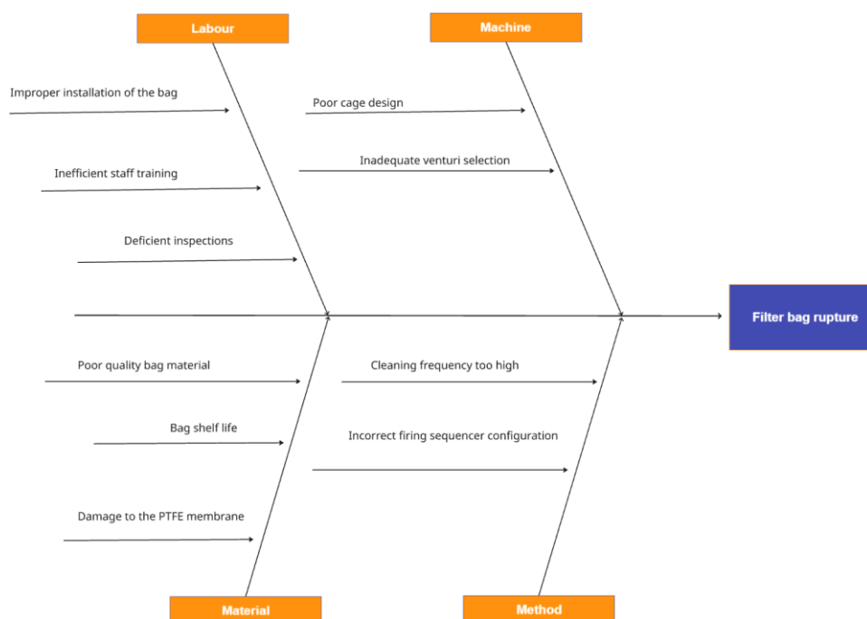
Figure 2. Ishikawa diagram for the analysis of causes of filter bag failure
